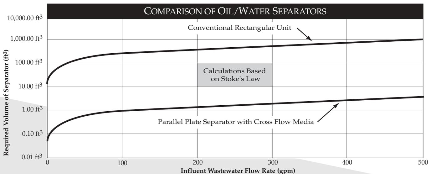
While packs with higher amounts of surface area can theoretically remove oil more efficiently, they may require more frequent maintenance. The angle of the plates should be somewhere between 45 and 60 degrees. Plate packs with 60 degree angles should be used if significant solids accumulation in the separator is anticipated.
